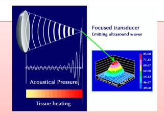
Acoustic lens concentrate multiple intersecting beams of ultrasound on a target in the body
